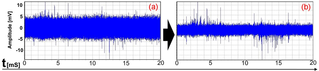
Figure 4 (a): Unfiltered 20 ms OLPD acquisition (b): Filtered 20 ms OLPD acquisition that shows PD peaks.
