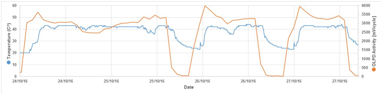
**Figure 2 Correlation between temperature and OLPD Activity on a 15 kV generator over a 4-day period .**
