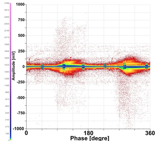
Figure 5 PRPD pattern produced from raw data before the de-noising process for U-Phase.
