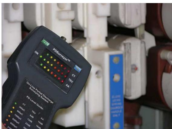
Figure 18: The PDSurveyor© Handheld PD Tester
