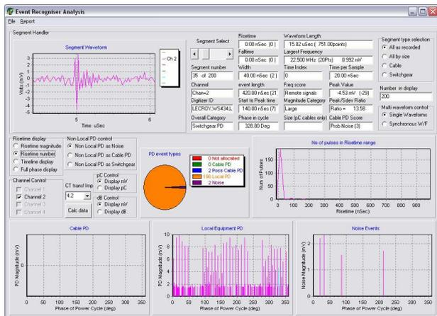
Figure 11 PDGold© Switchgear PD Event Recogniser Page
