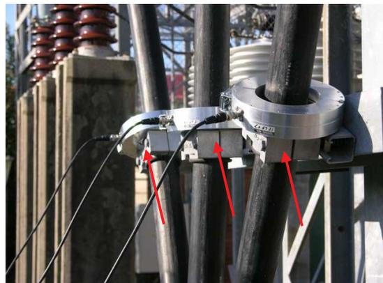
Figure 2: HFCTs around cores of 33kV XLPE cable
