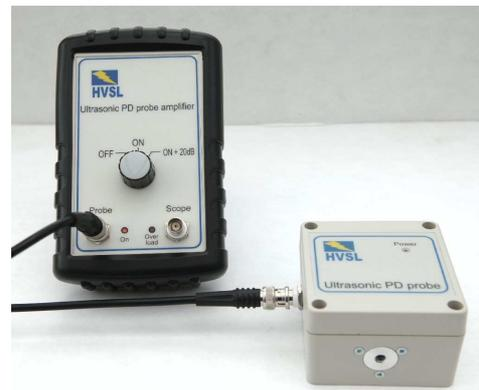
Figure 13: HVSL Ultrasonic PD Probe with Amplifier
