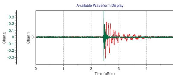
**Figure 14: 25kV VT PD pulse detected by TEV sensor (green) and HFCT (red) on**
