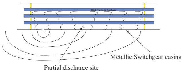
**Figure 8: Transient earth voltage radiation of PD**
