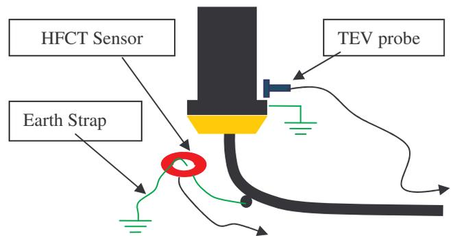
**Figure 16: Sensor Connection for HV Cable Testing**
