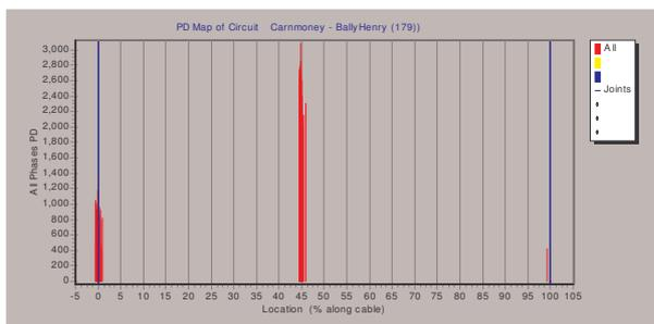
**Figure 7: PD Map of ‘mixed’ 33kV PILC/XLPE Cable**
