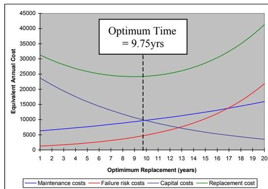
Figure 5: An Asset Management DSS for MV Plant
