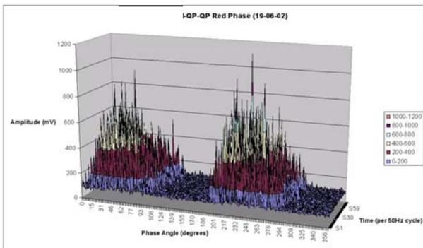
Figure 4a : PD Activity *before* joint replacement
