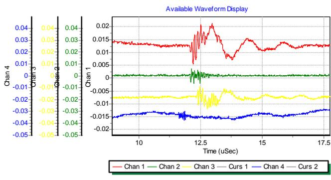
**Fig 3 Noise on various sensors on switchgear**
