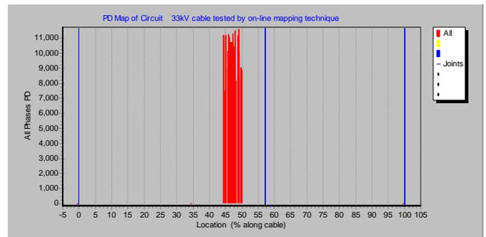
**Fig 6 On-line PD map of 33kV cable**
