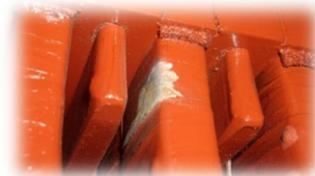
Figure 2. Surface discharge damage on rotating machine end windings
