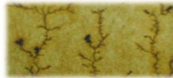
Figure 1. Tracking in Paper Insulation
