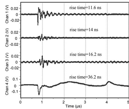
**Figure 5. Internal PD Pulse Waveform**
