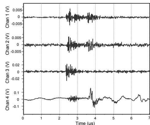
**Figure 6. Interfering PD Pulse Waveform**
