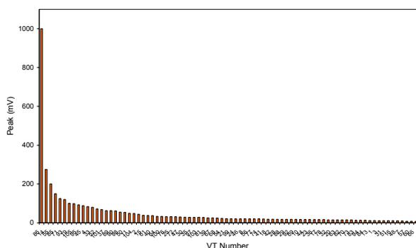
Figure 7 25kV Voltage Transformer PD Level Survey
