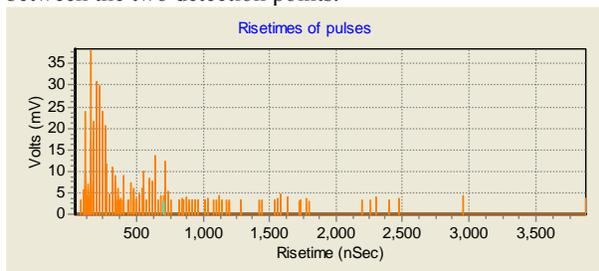
**Fig 3 Distribution of pulse risetimes from a cable**
