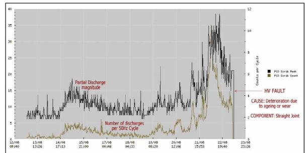
Figure 10: Partial Discharge trend immediately before failure.
