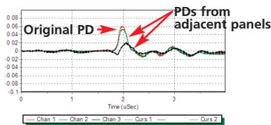
Figure 7: PD waveform captured on three adjacent panels.
