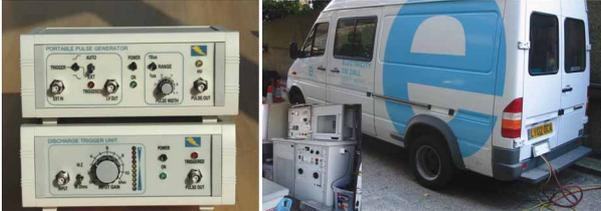
**Figure 12: Transponder and Off-line VLF testing equipment.**
