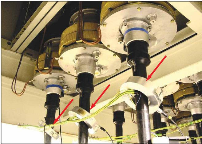
Figure 3: HFCT's around cores of 33kV XLPE cable
