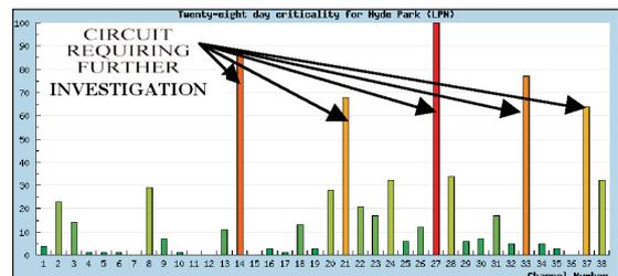
Figure 11: Cable ‘Criticality’ classification for a 38 Panel substation.
