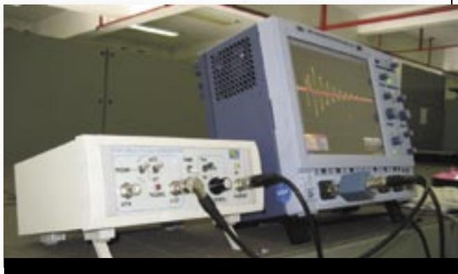
Fig. 1. The Portable Transponder and VLF testing equipment.
