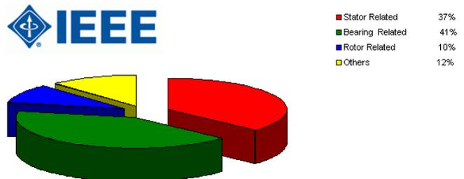
Figure 3. IEEE HV Motor Failure Causes Distribution [3]
