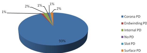
Figure 19: PD classification using Max AbsMin reduced matrix
