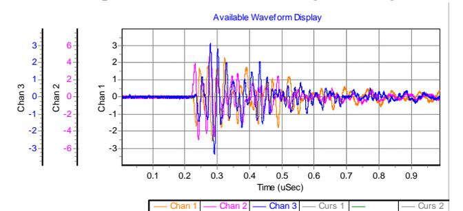
Figure 9. Type 1 PD: ‘Surface’ type PD event
