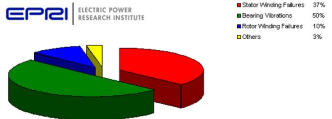
Figure 2. EPRI HV Motor Failure Causes Distribution [2]
