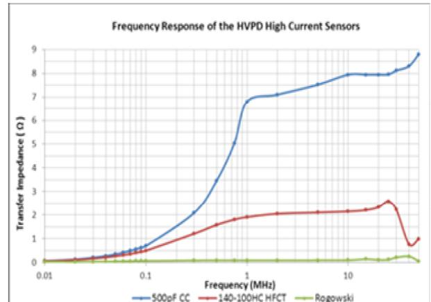
Figure 11. Frequency Response (10 kHz to 50MHz) for the 3 main types of Rotating Machine PD sensor
