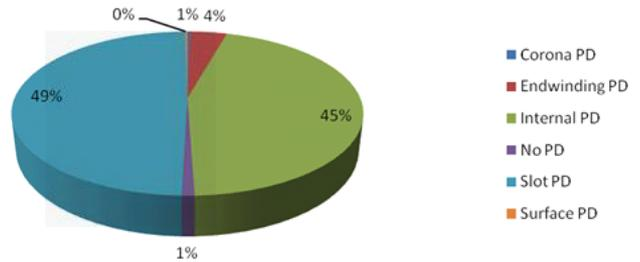
Figure 17: PD classification using Max\_Min reduced matrix
