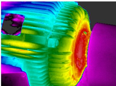
Figure 1. Overheated inboard bearing detected by infrared imaging
