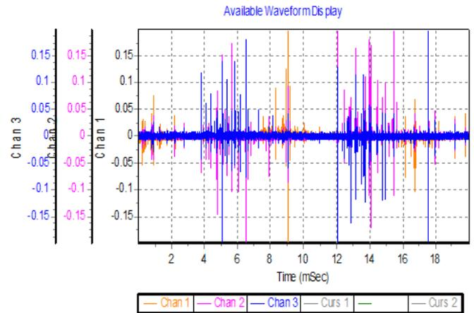
Figure 8. PRPD data from three phases of a hydro generator
