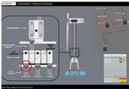
**Fig. 8 Turbine view – detailed PD, PQ and SC information is provided by Turbine, with alert levels.**
