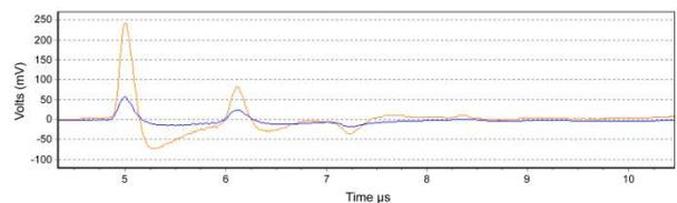
**Fig. 11: Partial Discharge pulse and the PD reflection (yellow phase) and the crosstalk on the blue phase**
