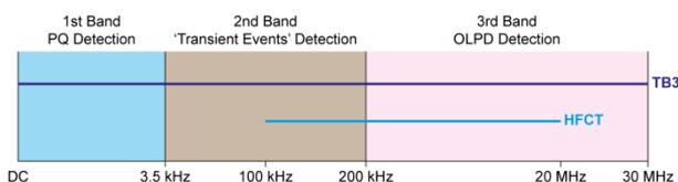
Fig. 4: The three (3) bands monitored by the TB-3 in comparison with the bandwidth of HFCT.
