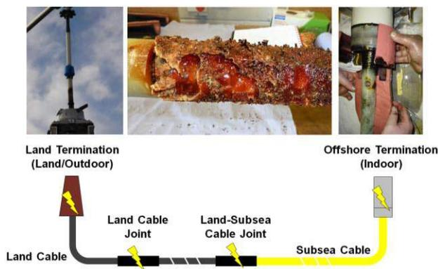
Fig. 2 Most likely sites of PD activity on subsea cables [6]
