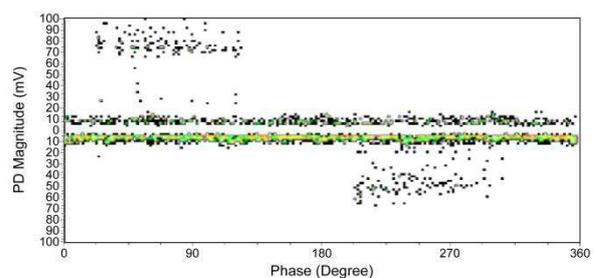
**Fig. 12: the PRPD pattern of the PD activity measured.**
