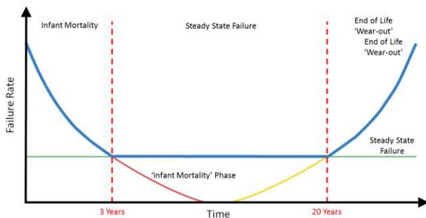
Fig. 1 The bath-tube curve
