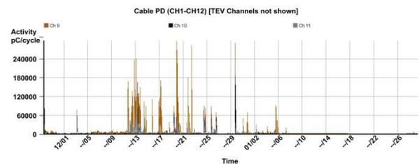
**Fig. 10: Intermittent PD activity (pC/cycle) detected over a 2-month period. Ch9: R Phase, Ch10: Y Phase, Ch11: B Phase**
