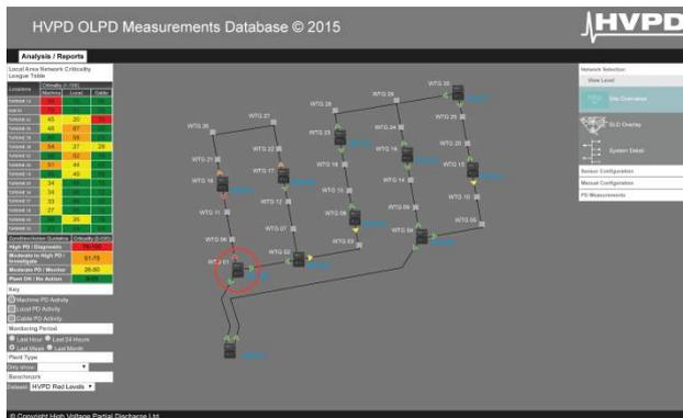
**Fig. 7 Top level overview – substations and turbines can be selected and viewed from central layouts**
