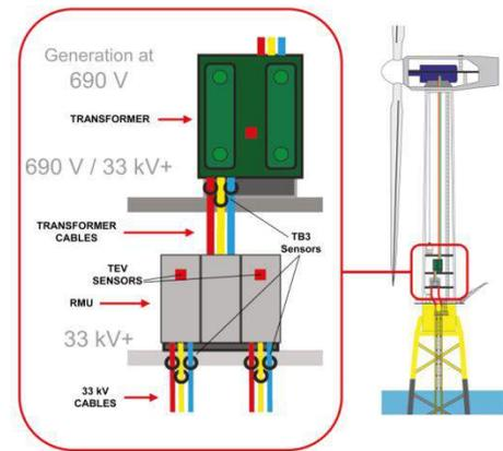
**Fig. 9: Installation of TB-3 sensors in an OWT**
