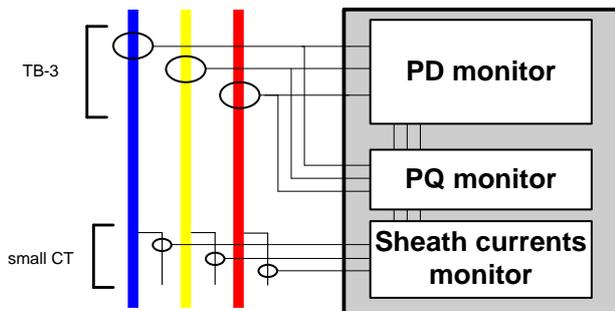
Fig. 3 HVPD OHVMS schematic of the functionalities and the use of TB-3 sensor
