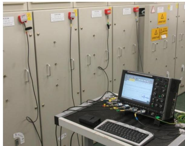
Fig. 5 Time of flight testing using 4x TEV sensors and Level 2 diagnostic test unit.
