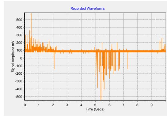
Figure 16 Generator 2 Line End 10kV PD phase pattern.
