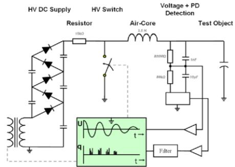
Figure 8 OWTS schematic [14].
