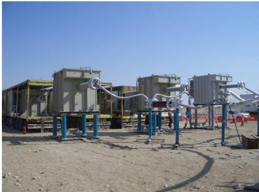
Figure 7 RTS to test a 400 kV line, 16 km long.
