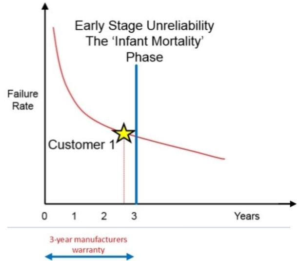
Figure 13 The ideal time for performing CM test of the assets in order to take full advantages of the manufacturer's warranty.
