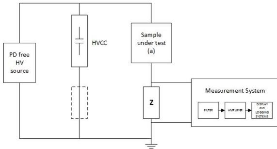
Figure 3 Basic diagram for electrical discharge detection [6]. In figure are clearly visible the HV PD-free source, the HV coupling capacitor, the sample under test (a) and the detection impedance Z; on the figure the alternative location for the Z is indicated with dashed lines.
