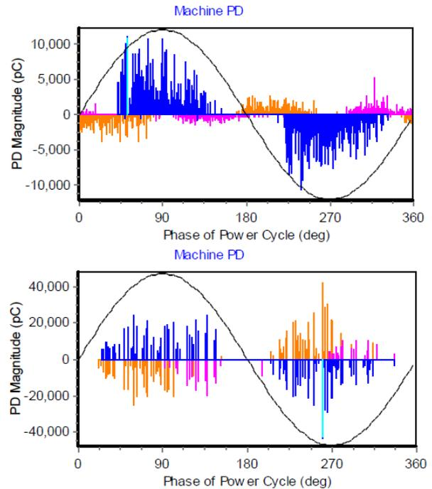
Figure 4 PRPD plots from PD measurements of rotating machines (motors). The figure on the top shows the Phase-to-Earth PD activity while the bottom one reports the Phase-to-Phase PD activity [7].
