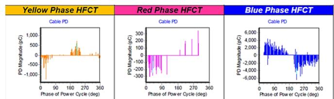
Figure 11 The on-line PD pattern detected within one of the cables.
