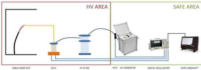
Figure 14 HVPD VLF test set.
