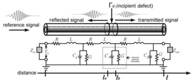
Figure 9 Transmission line model of a defect on a cable [15].
