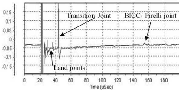
Figure 15 Details of the TDR measurement, in the picture are clearly visible the injected pulse and some of the reflected ones [16].
