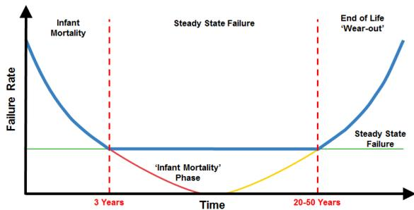
Figure 1 The "bathtub curve" base of the RCM [3].
