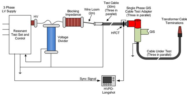
Figure 6 RTS test diagram.
