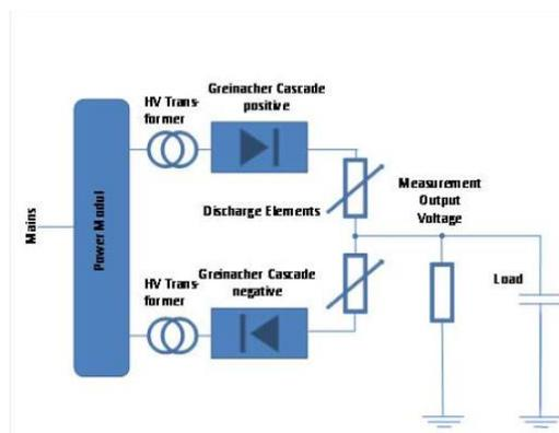
Figure 5 VLF voltage generation by controlled DC charging and discharging circuit [12].
