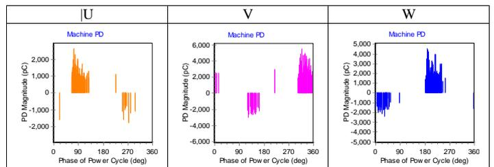
Figure 17 Generator 2 On-line PD phase pattern
