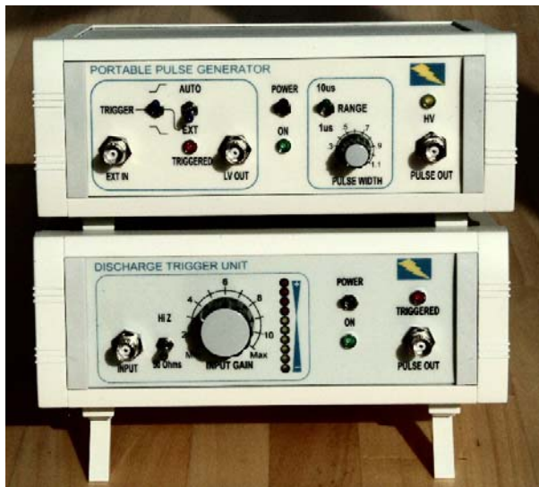
Figure 4 The trigger unit and large pulse generator of the transponder unit
