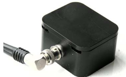
Figure 6 transient earth voltage probes (TEV's or capacitive pickups)
