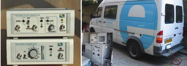
Figure 12: Transponder and Off-line VLF testing equipment.
