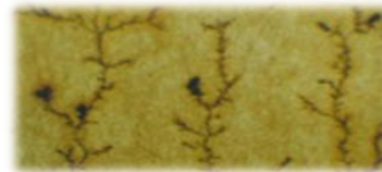
Figure 1. Tracking in Paper Insulation
