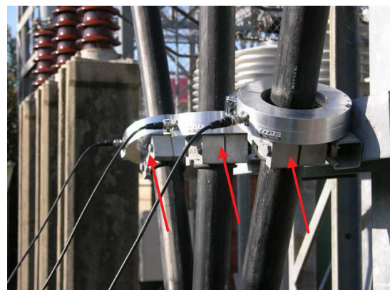
Figure 2: HFCTs around cores of 33kV XLPE cable
