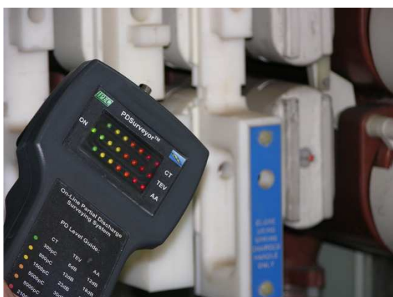
Figure 18: The PDSurveyor© Handheld PD Tester
