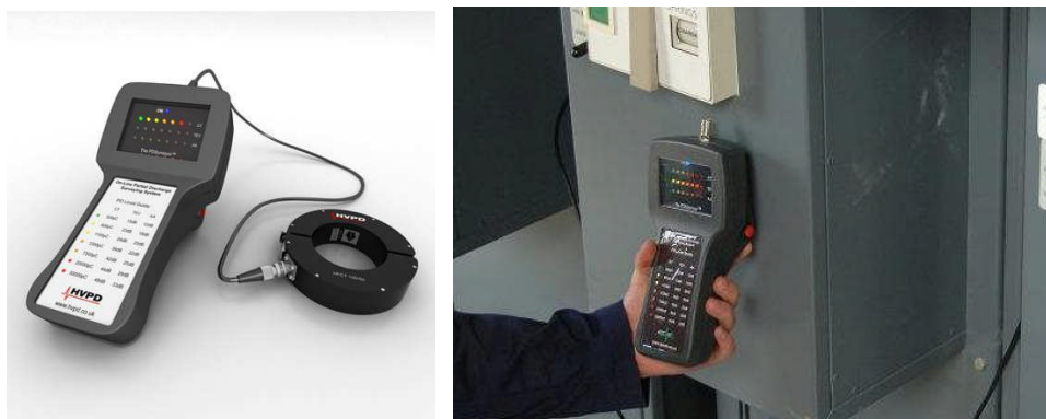
Figure 2: The HVPD PDSurveyor™ - TEV PD Detection on Cable Terminations and Switchgear
