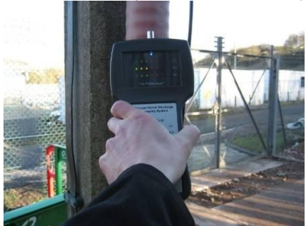
Low-Moderate TEV Activity as a result of Corona activity at termination
