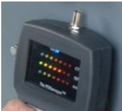
Figure 6: Panel 2 – PDSurveyor™ Display (RED 1 Level = 44 dB)
