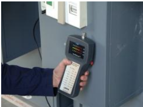
Figure 6: Panel 2 – PDSurveyor™ Display (RED 1 Level = 44 dB)
