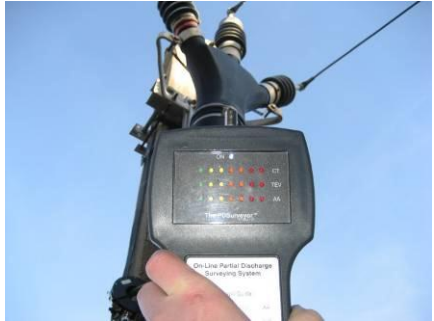
No Corona activity detected acoustically
