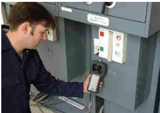
Figure 7: Panel 3 – PDSurveyor™ Display (YELLOW 2 Level = 28 dB)
