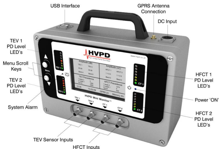
Figure 1: The HVPD-Mini™ Monitor 4-Channel PD Logger
