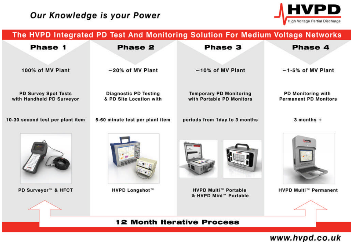
Figure 2: HVPD Solution for 4-Phase Asset Management Approach for On-line PD Testing and Monitoring of MV networks
